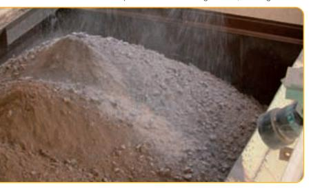
spray system. The system prevents the stone from being sprayed until it sees a full level, and also switches off spraying between wagons.
